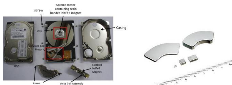
Figure 1. Sintered and resin bonded NdFeB magnets (left), voice coil actuator magnets used in a HDD (right) (Walton et al., 2015; www.techmetalsresearch.com )
