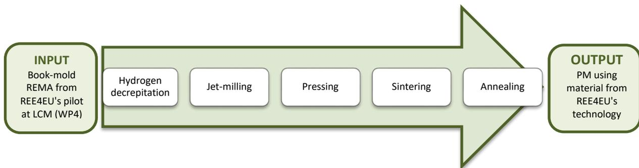
Figure 1. Schematics of the different steps followed in the manufacture of sintered NdFeB PM in the REE4EU project.
