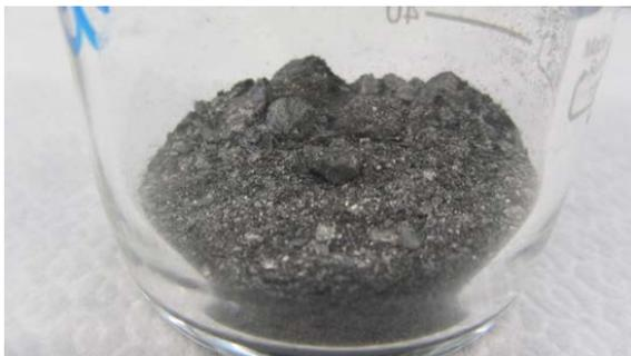
Figure 6. Coarse powder obtained after HD treatment of the long-duration annealed book-mold REMA block.
