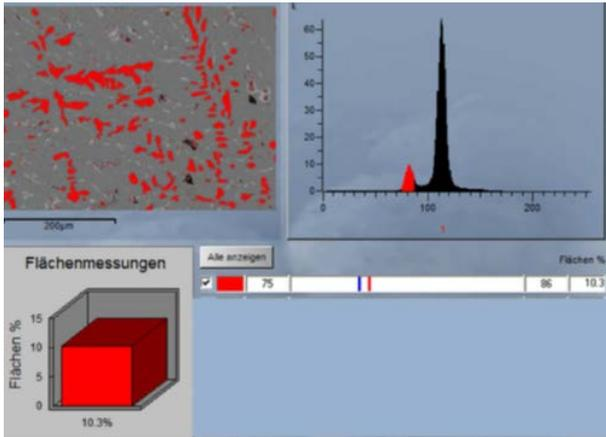
Figure 4. Metallographic determination of free Fe (marked in red).
