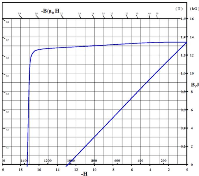
Figure 12. Demagnetization J(H)-curve of magnets from VAC mass production made from book-mold alloys with similar composition as the magnets obtained with the REE4EU's technology.
