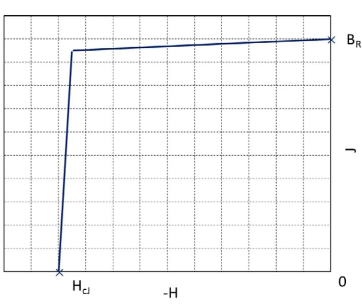
Figure 11. Example of determination of the remanence,  $B_R$ , and coercivity,  $H_{cJ}$ , from a demagnetization  $J(H)$  curve.
