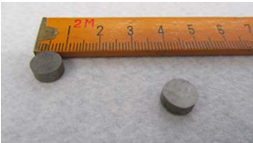
Figure 8. Examples of sintered PM obtained in the REE4EU project.
