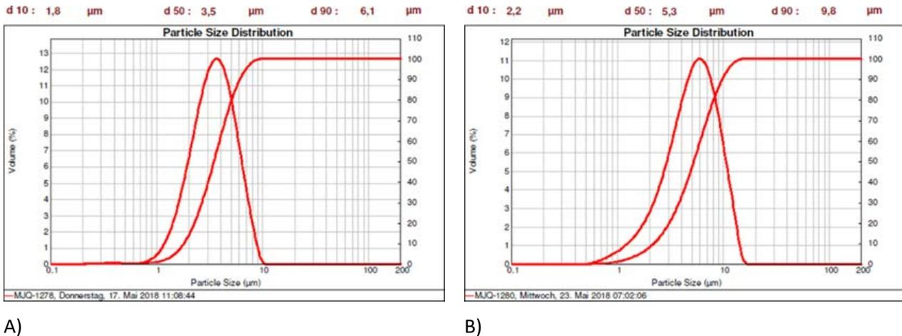
Figure 7. Particle size distributions of two batches of fine powders. A)  $D_{50} = 3,5 \mu\text{m}$ ; B)  $D_{50} = 5,3 \mu\text{m}$ .
