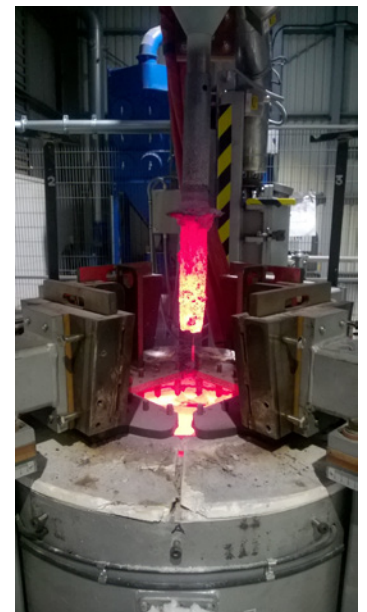
Trials of the pilot electrolysis cell at LCM
