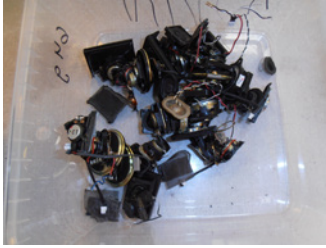
Loudspeaker element from EoL Laptops collected and separated at STENA
