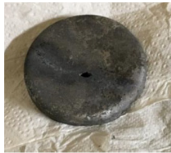
The REA alloy obtained, before and after re-melting to eliminate electrolyte remains
