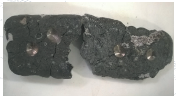
NdDyFe alloy produced in 1KA Pilot cell to validate the REE4EU technology
