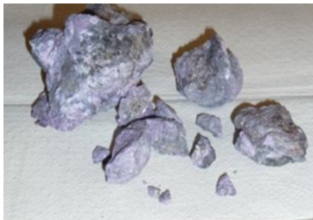
The REA alloy obtained, before and after re-melting to eliminate electrolyte remains
