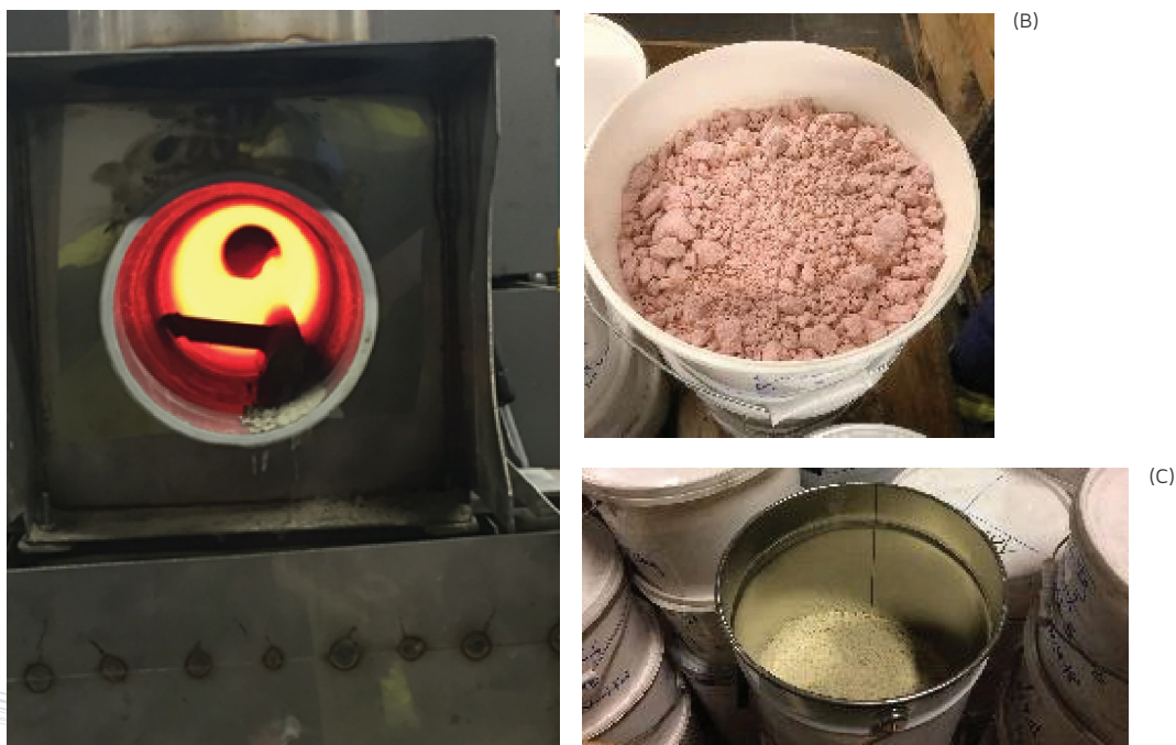
(A) The rotary kiln calciner, which uses (B) RE-oxalate mixtures from the ILE unit as input material, and gives (C) RE oxide mixtures as output material.
