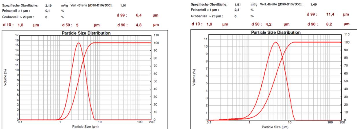
Figure 4. Particle size distribution of the two different powders ( $D_{50} = 3.0$  and  $4.2 \mu\text{m}$ )
