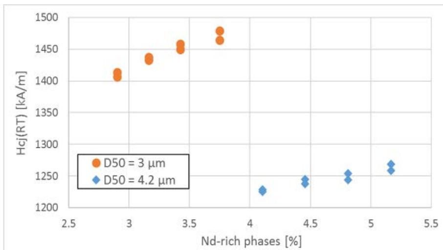
Figure 5. Dependence of the intrinsic coercivity  $H_{cJ}$  on the amount of Nd-rich phase in the magnet. Each of the measurements were carried out at two different sintering temperatures
