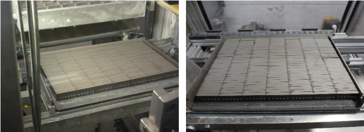
Figure 8. Pressed green bodies stored under inert  $\text{N}_2$  atmosphere
