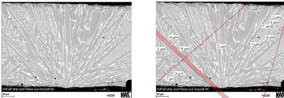
Figure 3. SEM micrographs of strip cast flakes. The figure on the right side shows the thicknesses of the lamellae
