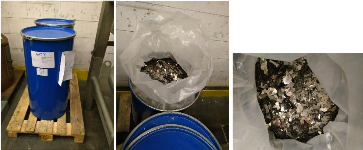
Figure 2. 600 kg strip cast flakes from LCM as received at VAC
