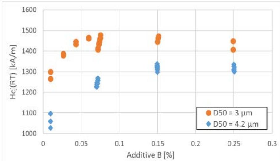
Figure 6. Dependence of the intrinsic coercivity  $H_{cJ}$  on the amount of B added during jet milling. Each of the measurements were carried out at two different sintering temperatures, the same as in Figure 5
