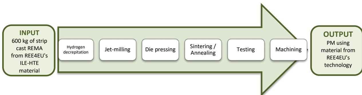
Figure 1. Schematics of the different steps followed in the manufacture of sintered NdFeB PM.
