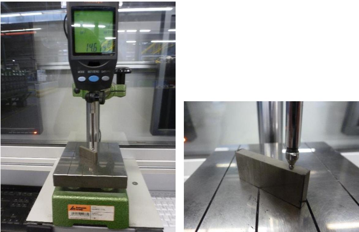
Figure 9. Dimension check of the green bodies directly after pressing
