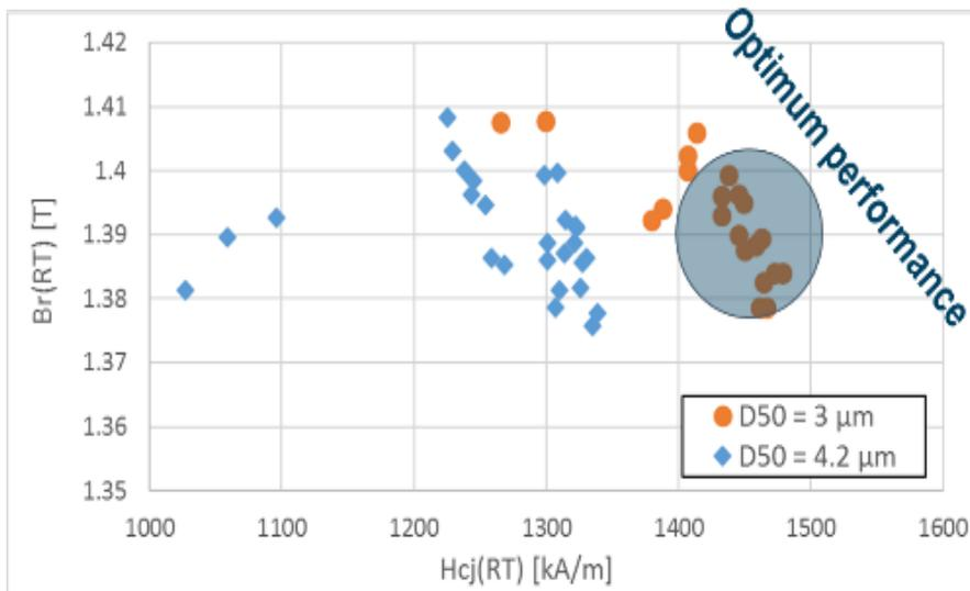
Figure 7. Relation between the remanence and coercivity for the different milling conditions that were investigated at the lab
